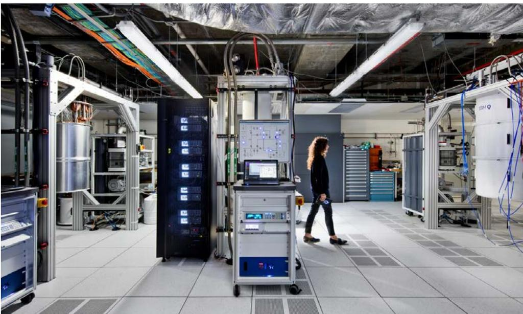
Inside the first IBM Q computation centre, dilution refrigerators with microwave electronics (middle) that operate IBM Q Network clients' cloud access to 20 qubit processor. (Credit: IBM/Connie Zhou)
